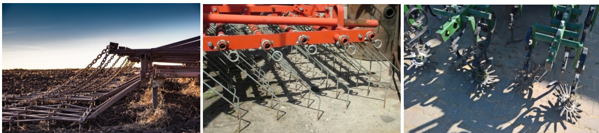
Figure 5.17 Harrows in weed management: chaine harrow (left - ( https://www.shutterstock.com ), tine weeder (middle – I. Tirczka), finger weeder (right – I. Tirczka)
